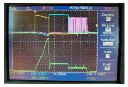
Fig 14. (c) Injection pulse signals and current waveforms of the GDI injector in the first driving pulse width (400µs)
