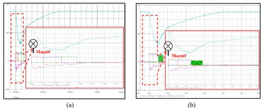
Fig 12. (a) Injection pulse signals and the GDI injector voltage and current waveforms without PWM control added to last pulse (I<sub>p1</sub>=400μs), (b) Injection pulse signals and the GDI injector voltage and current waveforms with PWM control added to last pulse (I<sub>p1</sub>=400μs)
