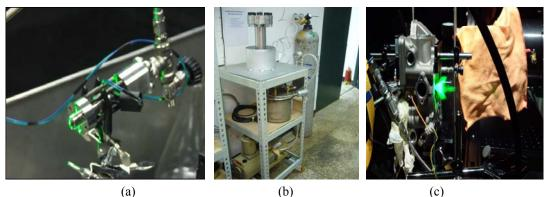
**Fig 2.** (a) The Bosch GDI single-hole injector test device, (b) High pressure 6~10 Mpa (Max) fuel supply system, (c) The test system of a Bosch GDI single-hole injector mounted on a 500cc motorbike engine cylinder head
