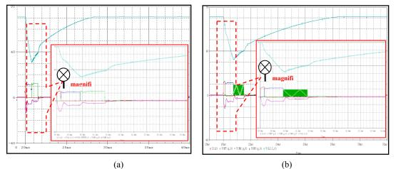
Fig 10. (a) Injection pulse signals and the GDI injector voltage and current waveforms without PWM control added to last pulse (I<sub>p1</sub>=120μs), (b) Injection pulse signals and the GDI injector voltage and current waveforms with PWM control added to last pulse (I<sub>p1</sub>=120μs)
