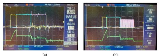
**Fig 13.** (a) Experimental driving pulse signals and GDI injector current waveforms without PWM control added to the last pulse (I<sub>p1</sub>=180μs), (b) Experimental driving pulse signals and GDI injector current waveforms with PWM control added to the last pulse (I<sub>p1</sub>=180μs)
