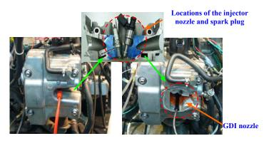
(b) (a) Figure 1. (a) Cylinder head of a PFI engine, (b) Cylinder head of a GDI engine
