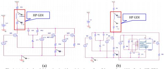
**Fig 4.** (a) A simulated drive circuit with an injection pulse of three pulse widths for the HP GDI Injector, (b) An improved drive circuit for the HP GDI Injector with three pulse and PWM control added to last pulse duration
