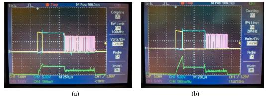
**Fig 14.** (a) Injection pulse signals and current waveforms of the GDI injector in the first driving pulse width (120µs), (b) Injection pulse signals and current waveforms of the GDI injector in the first driving pulse width (180µs)
