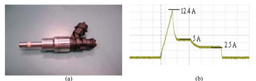
**Fig 3.** (a) A Bosch GDI single-hole injector, (b) Three pulse width operating current waveforms of the BOSCH GDI single-hole injector [7]
