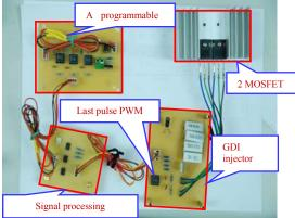
**Fig 6.** Practical implementation of the high-pressure GDI injector driving circuit board
