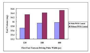
Fig 15. Effects of first fast turn-on driving pulse duration on the GDI injector fuel quantity
