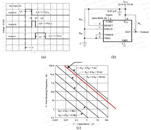
Fig 9. (a) Three different duration pulses and sequence [8], (b) PWM modulation circuit [8], (c) PWM operating frequency curves
