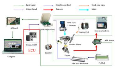
Fig 4. ECU configuration for 500cc motorbike engine
