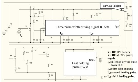
Fig 5. Electrical driving circuit diagram for the HP GDI Injector with three pulse width and PWM controller
