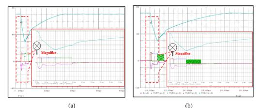
Fig 11. (a) Injection pulse signals and the GDI injector voltage and current waveforms without PWM control added to last pulse (I<sub>p1</sub>=180µs), (b) Injection pulse signals and the GDI injector voltage and current waveforms with PWM control added to last pulse (I<sub>p1</sub>=180µs)
